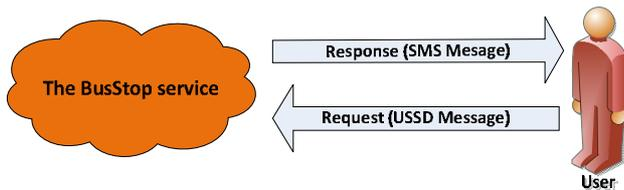
Fig 3. Functional schematic of the BusStop service
